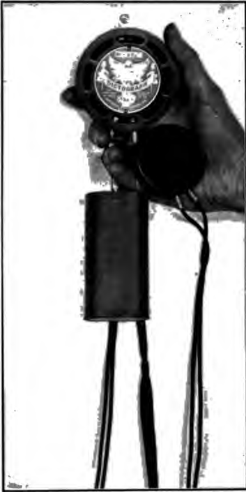
A COMPLETE DICTOGRAPH OUTFIT TRANSMITTER, EARPIECE, AND DRY BATTERY
