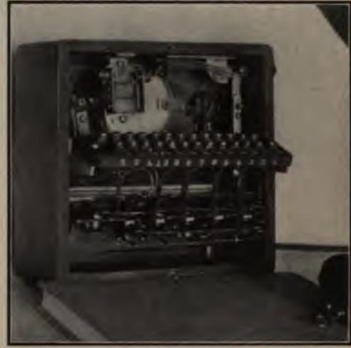
ONE OF THE PARENTS OF THE DETECTIVE DICTOGRAPH OUTSIDE AND INSIDE VIEW OF A TURNER TELEPHONE. EXPERIMENTS MADE TO PERFECT THIS DEVICE, THE COMMERCIAL DICTOGRAPH, AND THE ACOUSTICON, LED TO THE DEVELOPMENT OF THE DETECTIVE APPARATUS
