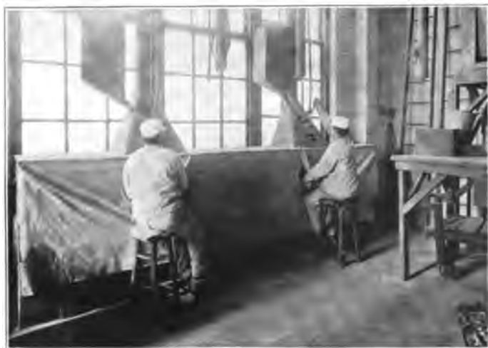
Sand blasting the brass trimmings of the car before applying the finish
