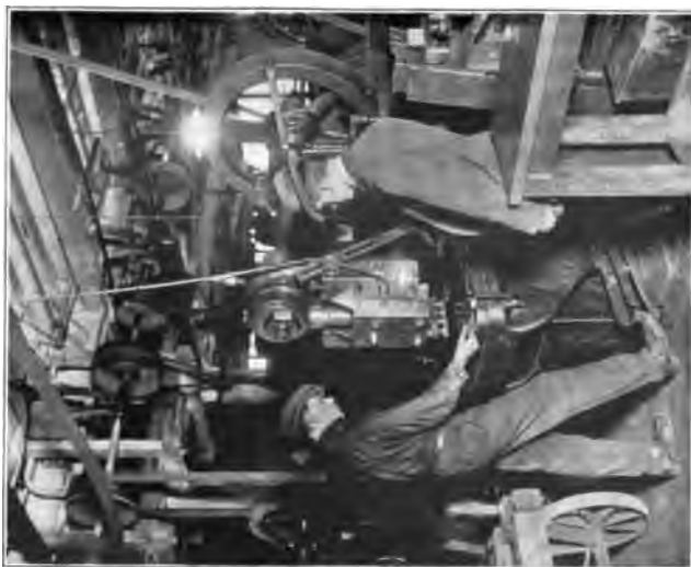
This machine is at work punching holes for screws etc. in the steel for the inside finish
