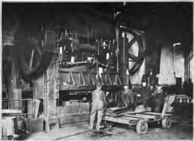
Another large press at work on the forming of steel shapes for the interior framing of the cars
