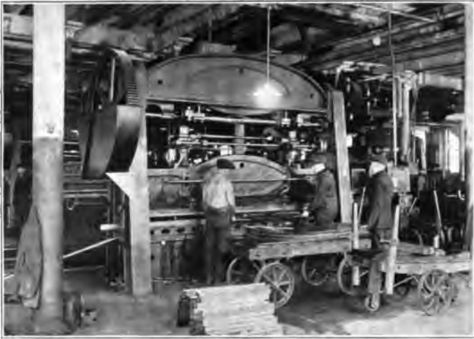
The steel parts used for interior car finish are all standardized, and are formed by powerful presses
