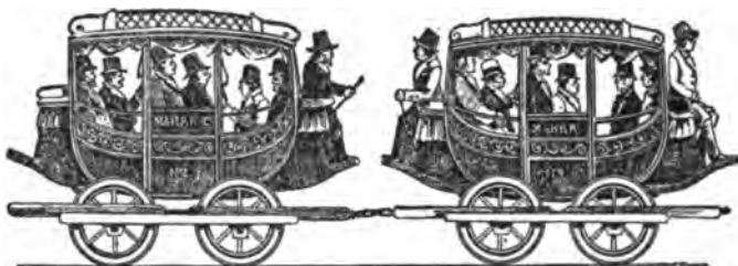
Early passenger cars, designed after the then prevalent type of horse coach. These cars were part of the train that ran on the formal opening of the Mohawk & Hudson Railroad (the first link of the New York Central System) on July 5, 1831.
