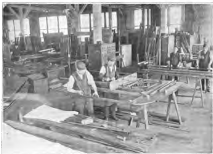
The assembling of the steel car partitions is shown in this picture
